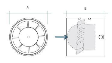
To be installed in rigid or flexible ducts  $\emptyset$  100 mm and  $\emptyset$  125 mm. You can join AA100T tube with  $\emptyset$  100 mm tube using CG100B joint.
