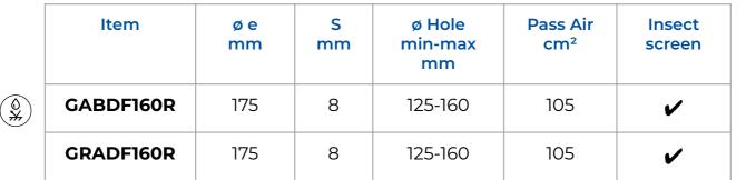
**Description:** Foldable ventilation grille with fixing springs
